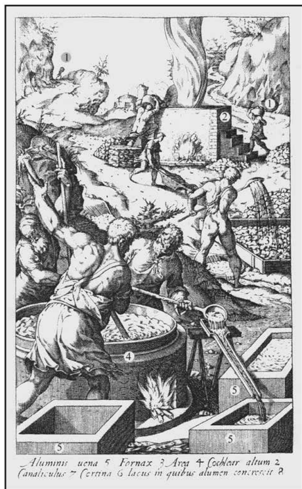
Fig. 245. Copperplate engraving depicting the manufacture of alum in Tolfa during the 18th century. 1) transport of alunite to the processing site; 2) calcination kiln; 3) rinsing of the raw material; 4) boiling of the alum mass and 5) crystallization caisson (illustration after Mercatis 1719, 55).
