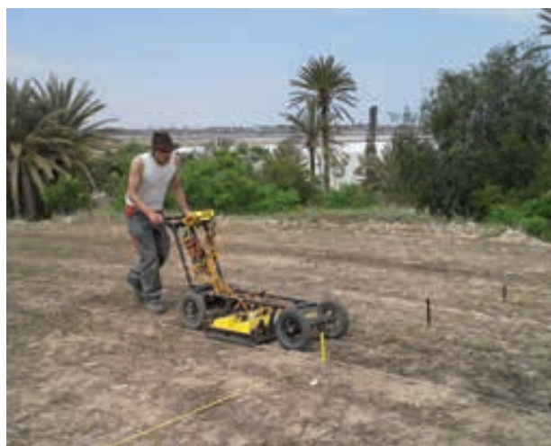
Fig. 34. GPR measurements in Area A with the three-channel 500 MHz system.
