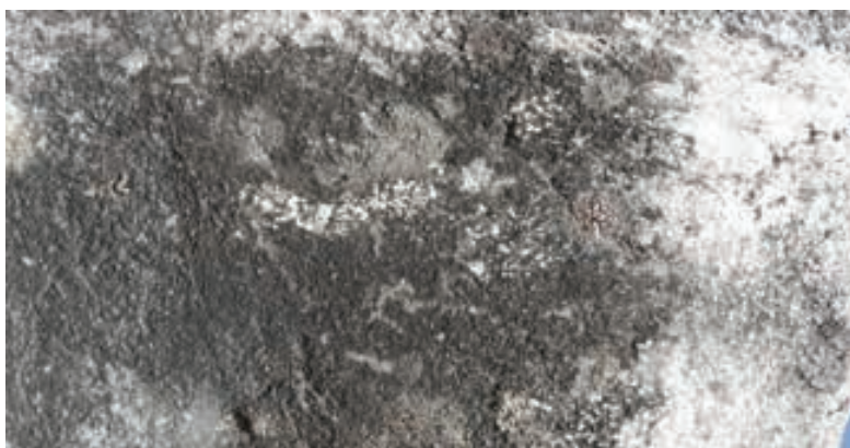
Fig. 36. Biodiversity on marble: cyanobacteria enter between the crystals and give a black hue to the stone.
