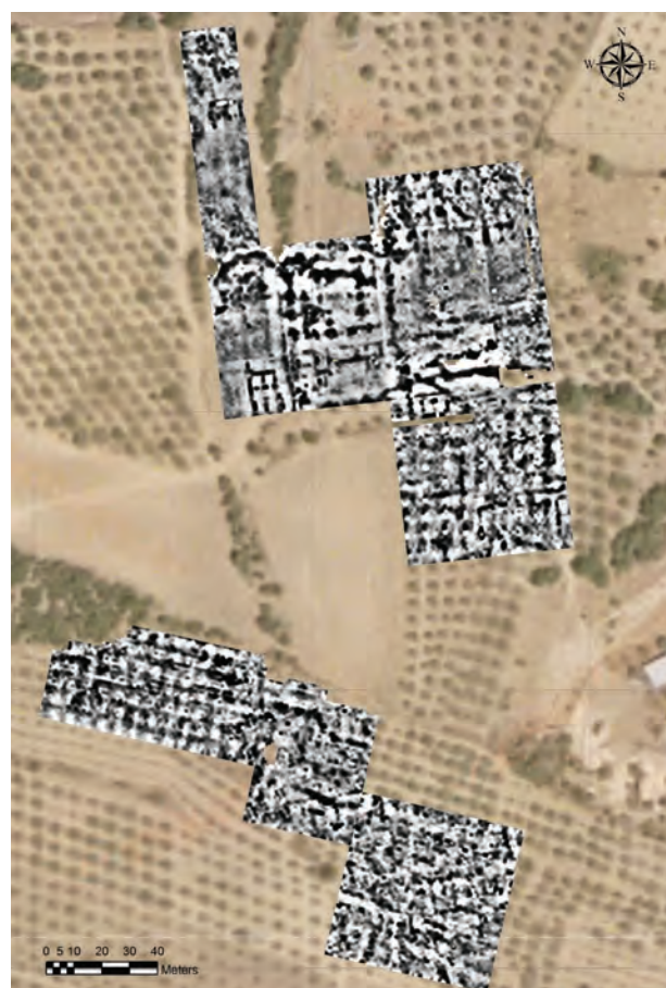
Fig. 11. Distribution of the resistance in the same area as in Figure 10 after the application of Wallis filter.
