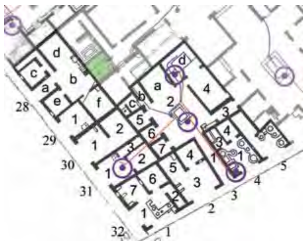
Fig. 27. Plan showing the southwest part of insula V 1, with waterlines, inlets in blue, drains in red. Kitchen of the Casa del Torello in green. After CTP IIIA. By Henrik Boman.
