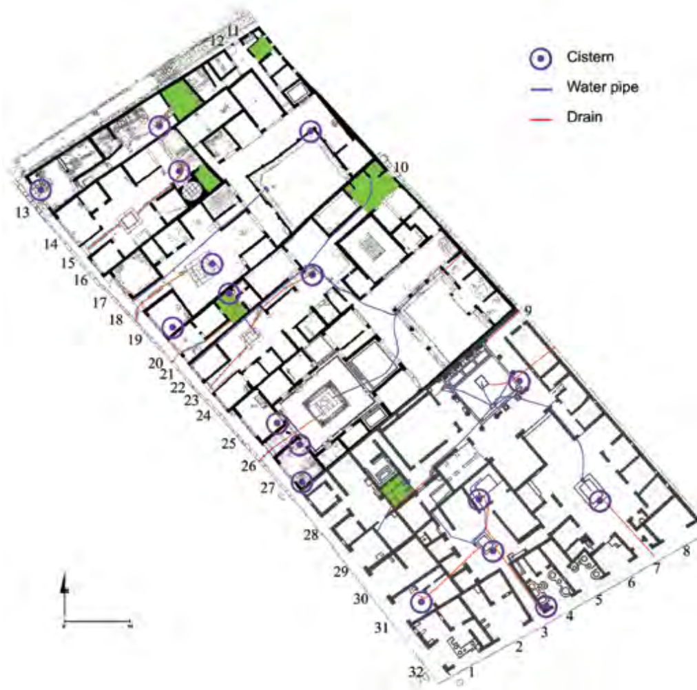
Fig. 14. Water pipes and cisterns in insula V 1. Blue lines used for inlets, red for drains; kitchen areas in green. By Henrik Boman.
